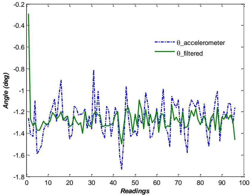
Figure 3. Filtered vs accelerometer data in a static position
