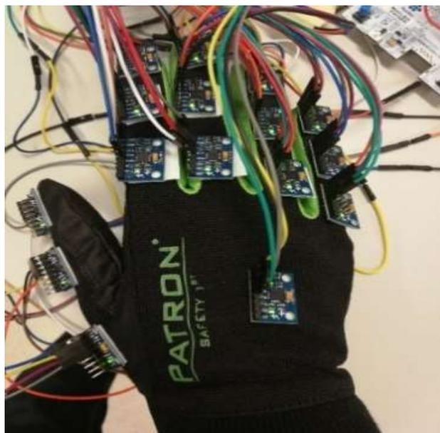
Figure 2. Glove prototype with 16 MPU-6050
